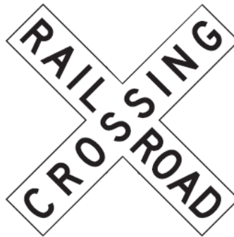
Figure 29. Railroad crossbuck sign. Source: MUTCD
