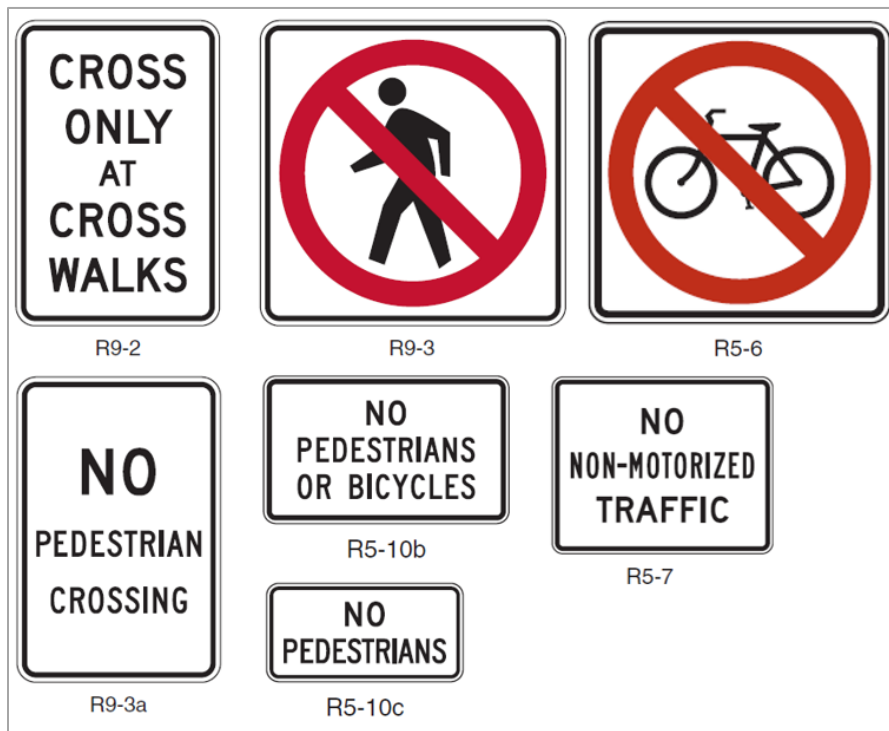
Figure 34. Examples of non-motorist prohibited signs. Source: Manual on Uniform Traffic Control Devices (MUTCD), FHWA
